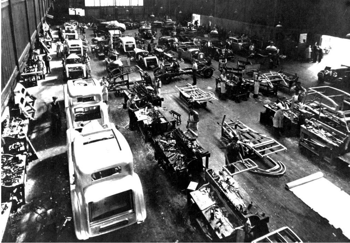
The Vanden Plas coach-building works in full production, around 1930, showing the craftsmen, each with his own bench, carrying out the stages of building different car bodies on a variety of chassis.
